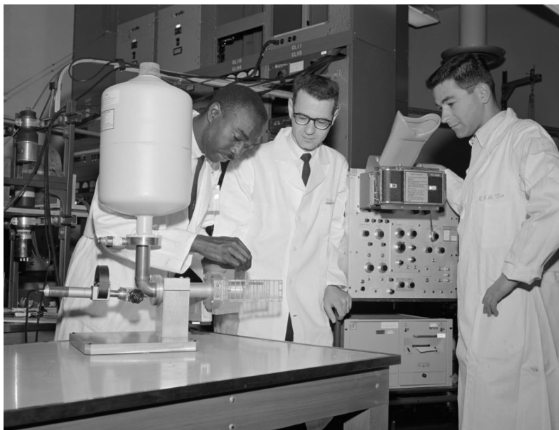
Figure 4. James Harris (left), Jack Hollander (middle), and Stanley Prussin (right) with their germanium–lithium gamma ray detector used for detecting impurities with neutron activation analysis, 1965. Photo courtesy of Lawrence Berkeley National Laboratory. ( https://photos.lbl.gov/bp/#/search/4605505?q=James%20Harris&filters=%257B%257D ).
